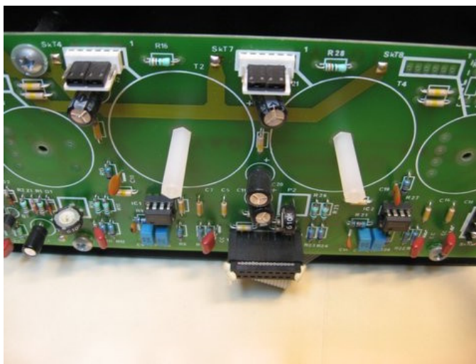
The Nylon mounting posts fitted in place. The screws are firm but not tight.
