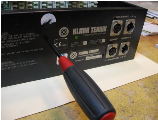
Above shows fitting the Nylon screws from the rear
