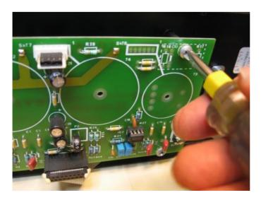
Undo the four screws on the PCB with a stubby screwdriver.
