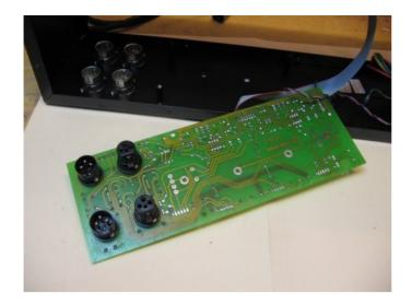
Re-solder the bypass relays and anything suspect looking in the area. Only use good quality standard 60/40 solder. Pay particular attention to the pins that connect the top side of the circuit board to the bottom side.
