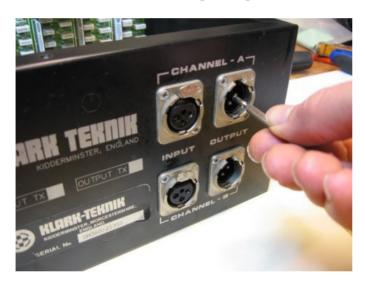
First unlock the latches in each XLR connector with a jewellers screwdriver. The latches are released with a small turn anticlockwise, be gentle with the latches.
