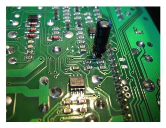
Fit a 105 degree 10uF 25 volt electrolytic capacitor where the SMD capacitor was, the negative pin faces the control card pins (right hand side of this image).
