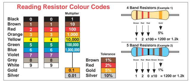
A resistor will limit the current flow through itself to a calculable value based upon its resistance and the applied voltage (see Ohm's Law). This means a resistor can be used to run a low voltage device from a higher voltage supply by limiting the required power to a predetermined level. Resistors are not polarity sensitive.
