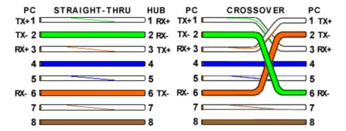
Note that pins 4, 5, 7, and 8 and the blue and brown pairs are not used in either standard. Quite contrary to what you may read elsewhere, these pins and wires are not used or required to implement 100BASE-TX duplexing--they are just plain wasted.
